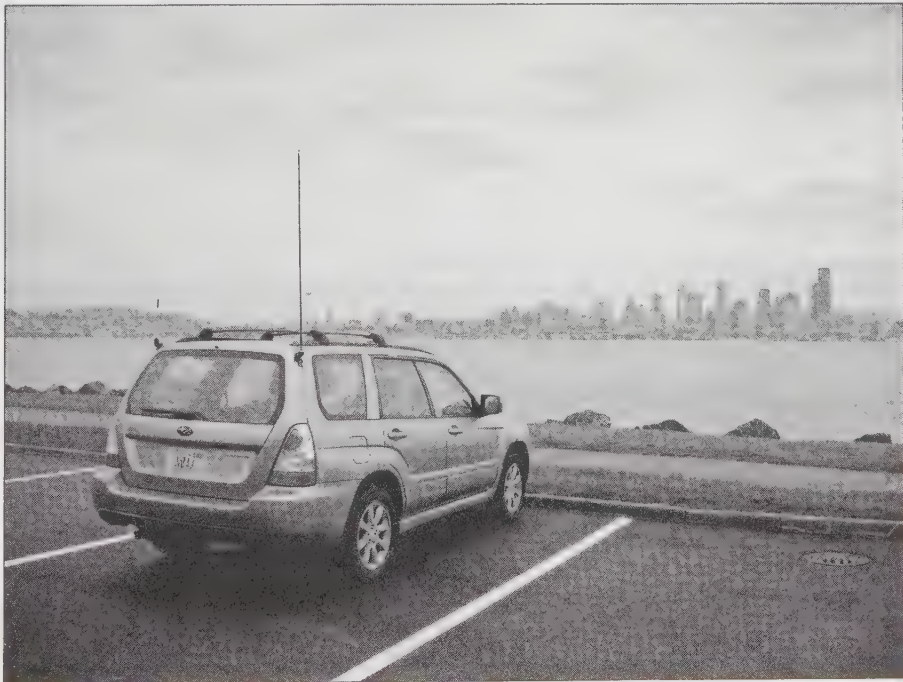
Figure 12-5: A Hamstick-type mobile antenna mounted on the NØAX mobile along with a small VHF/UHF dual-band whip.
