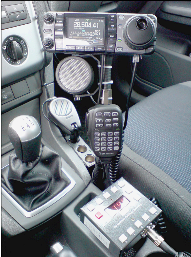
Figure 13-6: Clever use of flexible mounts and cupholders makes for a compact mobile station.
