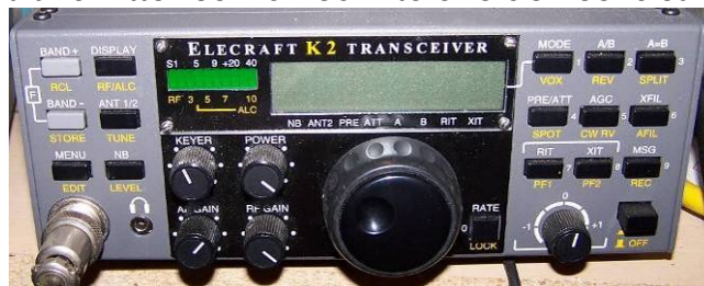
Figure 27 - Elecraft K2 HF Transceiver. Photo by N5IUT
