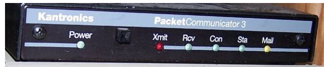
Figure 34 - A Kantronics KPC-3 TNC. Photo by N5IUT
