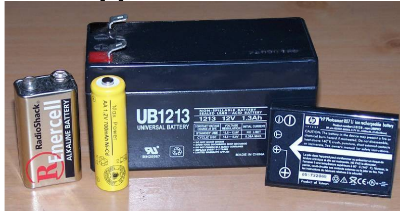
Figure 25 – Displayed from Left to Right is a 9 Volt Alkaline, a 12 Volt 1.3 Amp/hour Sealed Lead Acid, a 1.2 Volt Nickel-cadmium size AA and a 7.3 Volt 1 Amp/Hour Lithium-ion camera battery. Photo by N5IUT
