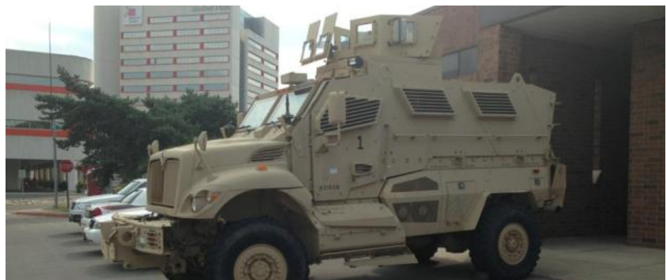
The Ohio State University MRAP was "built to withstand ballistic arms fire, mine blasts, IEDs, and Nuclear, Biological and Chemical environments that threaten the safety of its crew."
