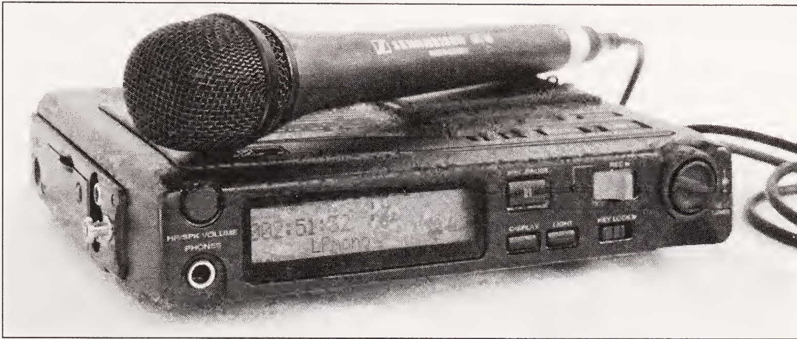
Figure 5-12. Marantz PMD 670 and Sennheiser MD46 mic (Photo © 2005 Jason Niedle)
