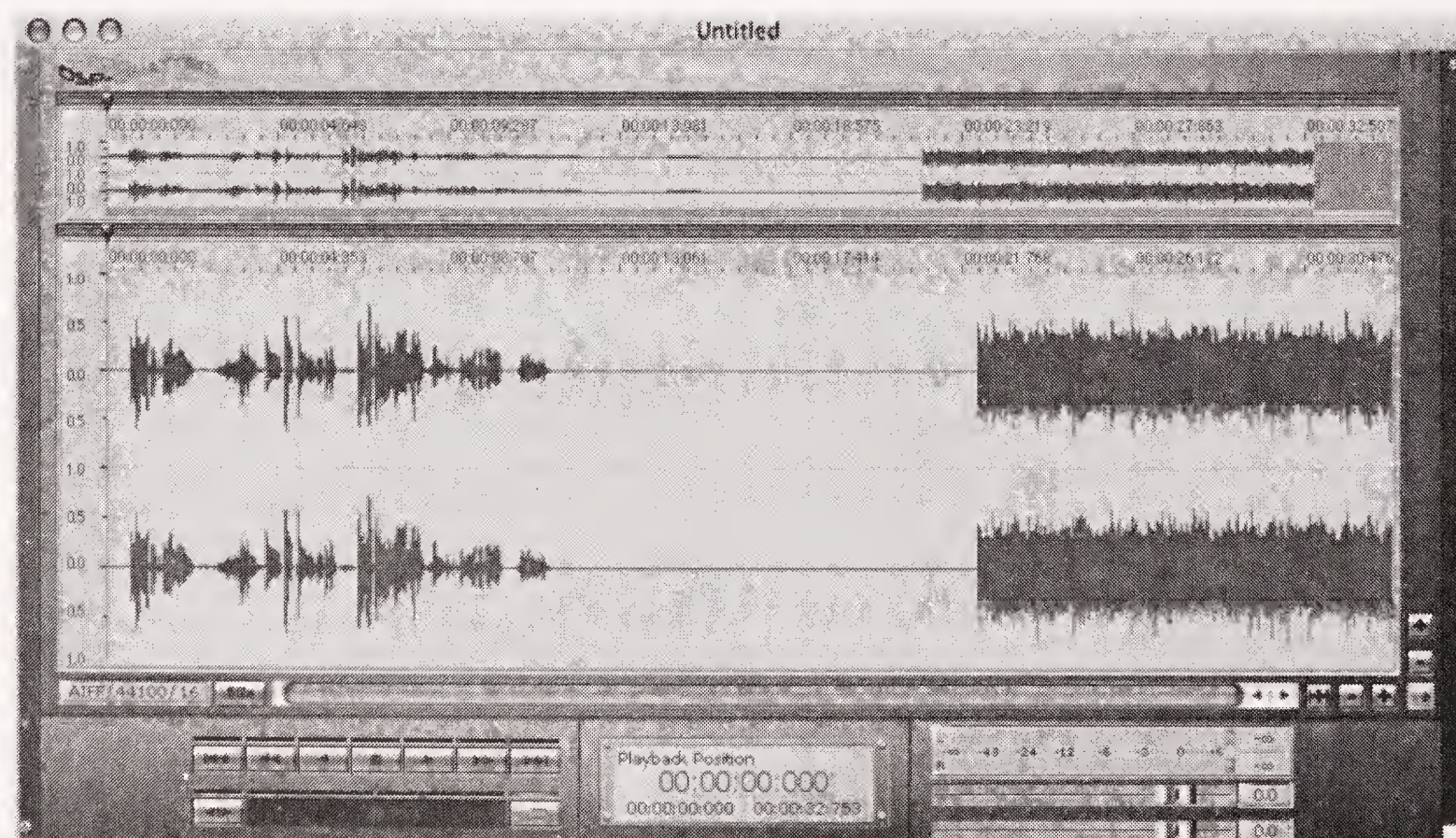
Figure 6-1. Sample waveforms, with a section of speaking, a section of silence, and a section of loud music (in the application DSP-Quattro)
