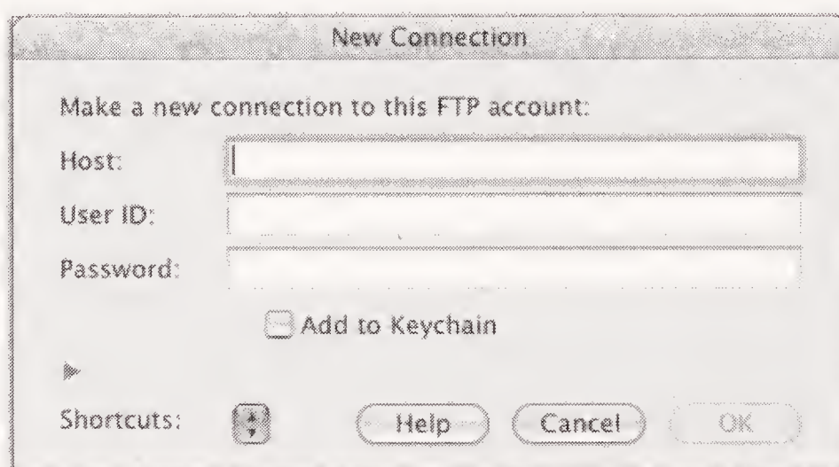
Figure 9-1. The New Connection window in Fetch. All FTP clients will ask you for the same basic information: host, user ID/username, and password.
