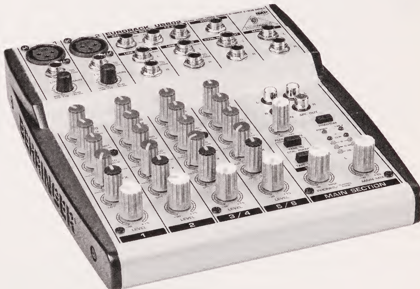
Figure 2-4: The Behringer Eurorack UB802 Mixer, a simple mixing board, accommodates two phantom-powered microphones and jacks for live instruments.
