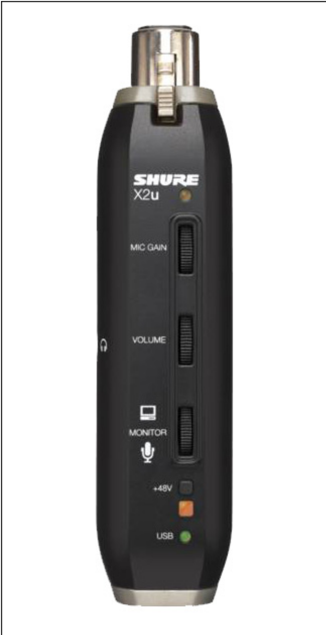
FIGURE 11-4: Turn any XLR microphone into a USB mic and control the strength of your mic signal with the Shure X2U XLR-to-USB adapter.
