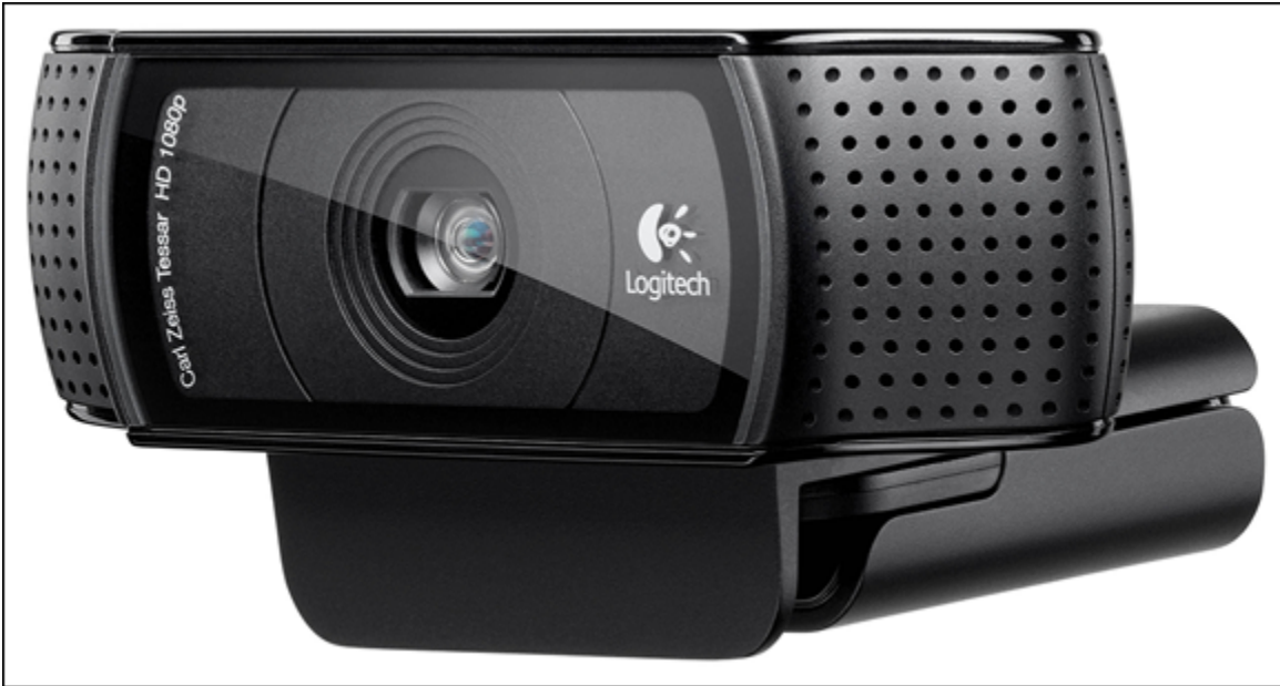
FIGURE 6-10: The Logitech C920 webcam, priced at just under $50, offers streamers full 1080p video, built-in microphones with automatic noise reduction, and automatic low-light correction.
