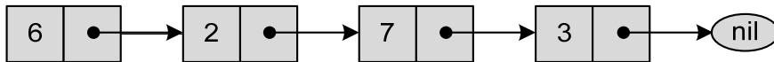
Figure 3.1 Functional list containing 6, 2, 7 and 3. Rectangle represents cons cell, which contains a value and a reference to the rest of the list. Last cons cell references a special value representing an empty list.
