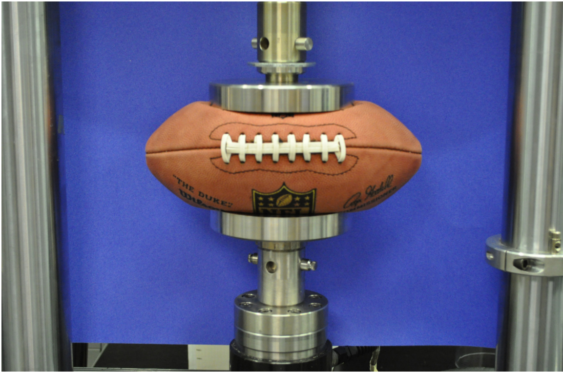
Figure 15. A photograph of the football being subjected to 650 pound cyclic loading. Note the overall deformation of the football.
