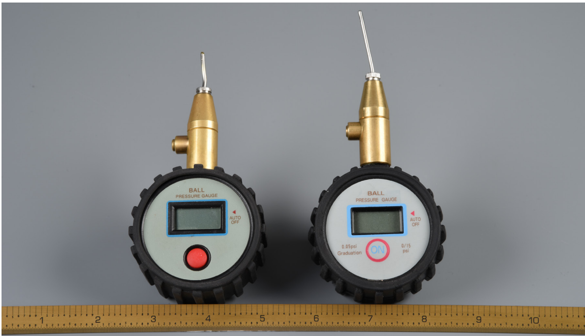
Figure 2. Image showing the front of the Non-Logo Gauge (left) and Logo Gauge (right).
