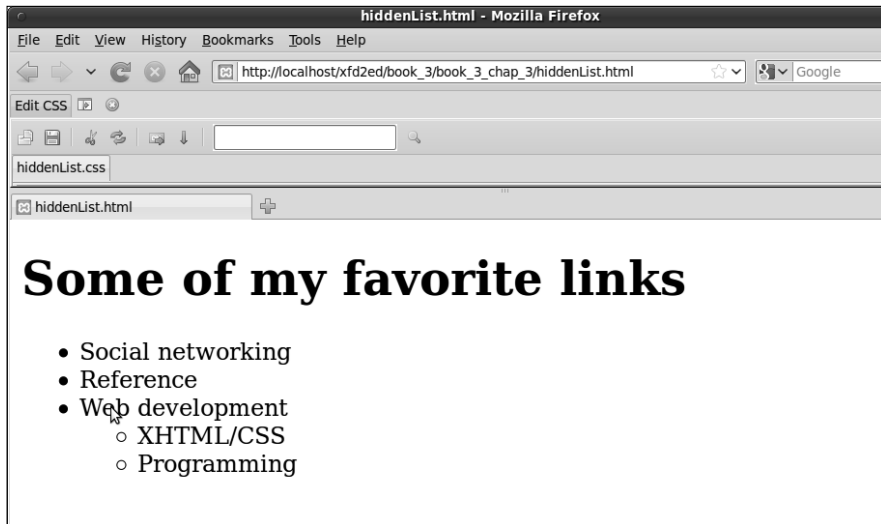
Figure 3-7: Now, only the next menu level shows up on a mouse hover.
