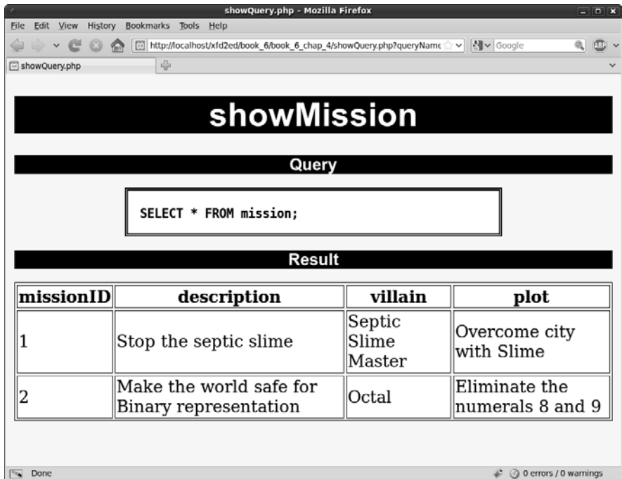
Figure 4-10: The mission table handles mission data but has no link to the hero.
