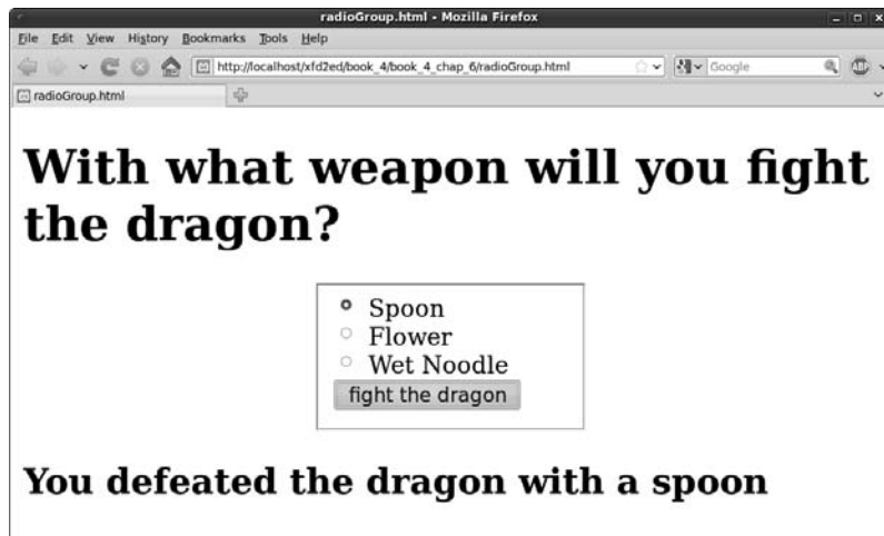
Figure 6-4: One and only one member of a radio group can be selected at one time.
